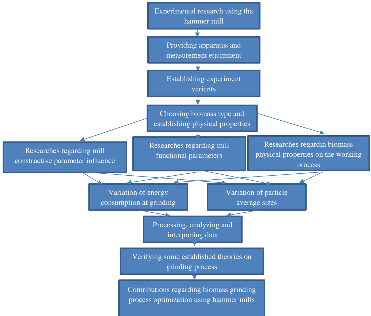
Fig. 5.12. Experiment course schema for analyzing hammer mills working process
